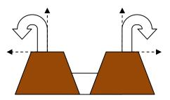
Bending Shows exaggerated elongation at top and shortening at bottom of ridge before eventual brittle failure
