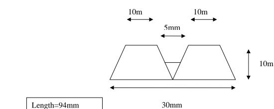
The shape is above undergraduate level so I shall work out the moment of inertia for one finger. Using the above formula and approximate dimensions a,c,d=10mm and b=15mm give the second moment of area to be  $I_{xx}$ =3403mm<sup>4</sup>.
