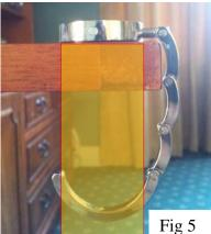
The base covers a cross sectional width which can be seen to be the safe zone for loading. As long as the load applied is under this area, the base will not lift or slide.
