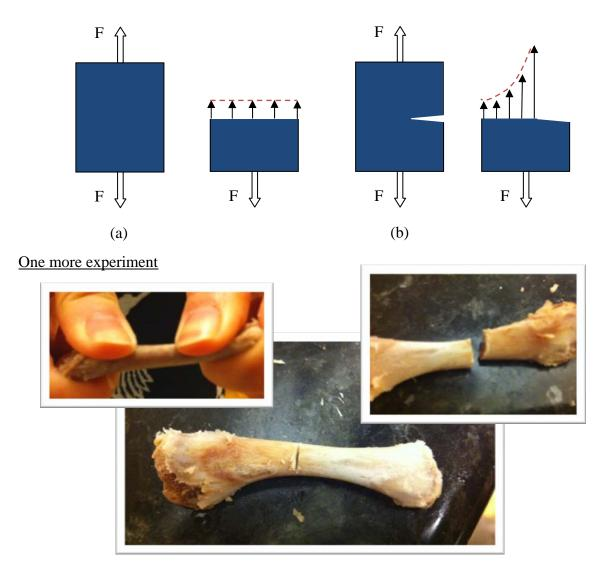
People in China like eating Sparerib Soup, while the ribs are difficult to cut off and snap (see above). A common method to deal with this problem is to use knife to make a crack on the bone. It can be found that just a small bending moment can break the bone into two pieces. Obviously, the crack gives rise to the stress concentration (the stress is higher near the crack than that in other parts of the bone), so it is easy to break the bone.
