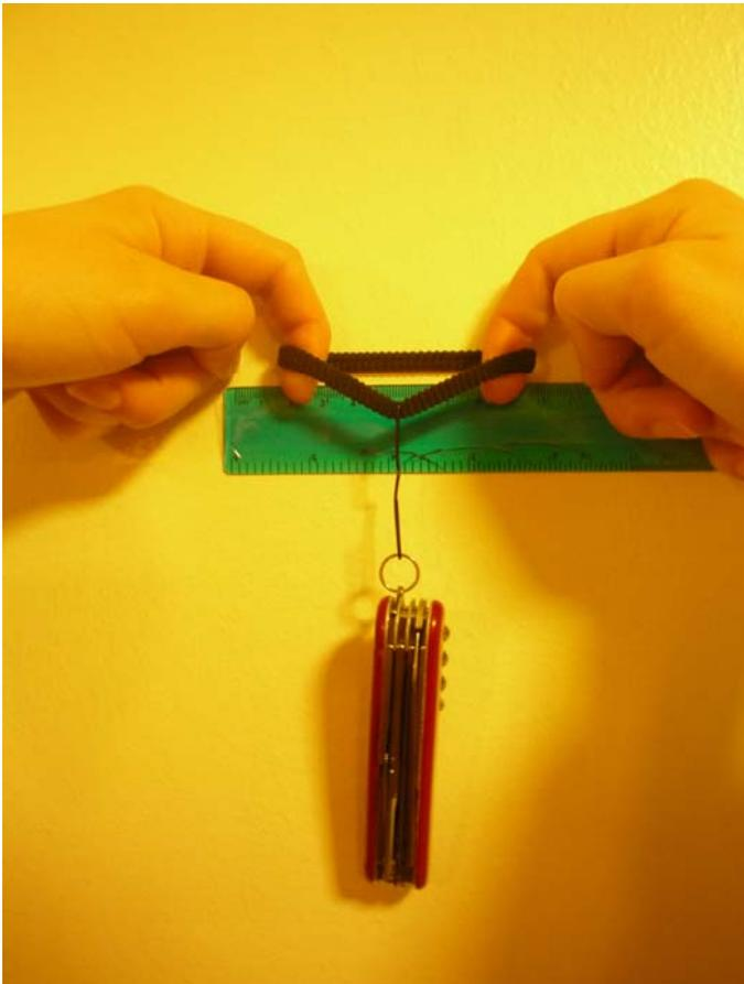
A hair band spanning a distance of 5cm. Hair band is loosely held in place. A concentrated load is applied at midspan, causing considerable deflection.
