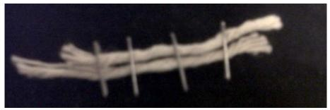
Figure 1: Stapled reinforcement string used in ice beam (2)
