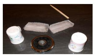
Figure 3 – Ice beam (1) failed under load of 1.25 kg
