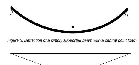
Figure 6: Bending Moment Diagram - simply supported beam with point load in centre
