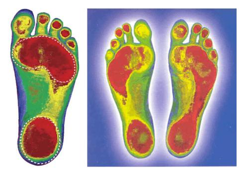
These pictures show the foot surface where test have been done in order to check the weight distribution on to our foot. The red section shows that the area with highest force exerted and the green section are the least force exerted by the human. This shows that different parts of our foot surface will have different amount of force exerted onto the floor while in standing stance.
