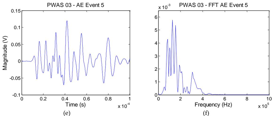
350 **Figure 12.** Typical experimental AE waveforms and Fourier Transform from a transverse crack in
