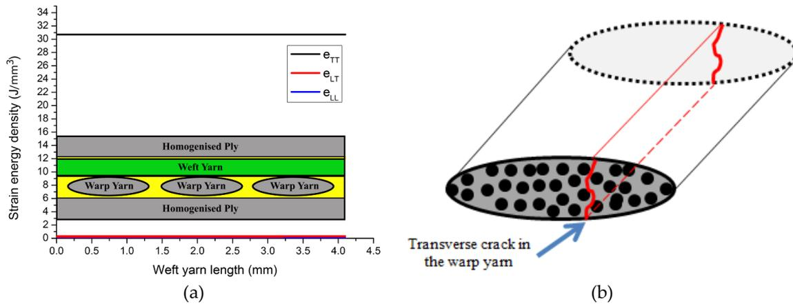
223 **Figure 4.** (a) Strain energy release rate along weft yarn (TT: Transverse component; LT: shear
