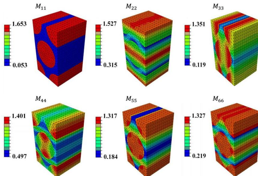
Figure 16. Diagonal elements of SAF tensor for hexagonal unit cell.
