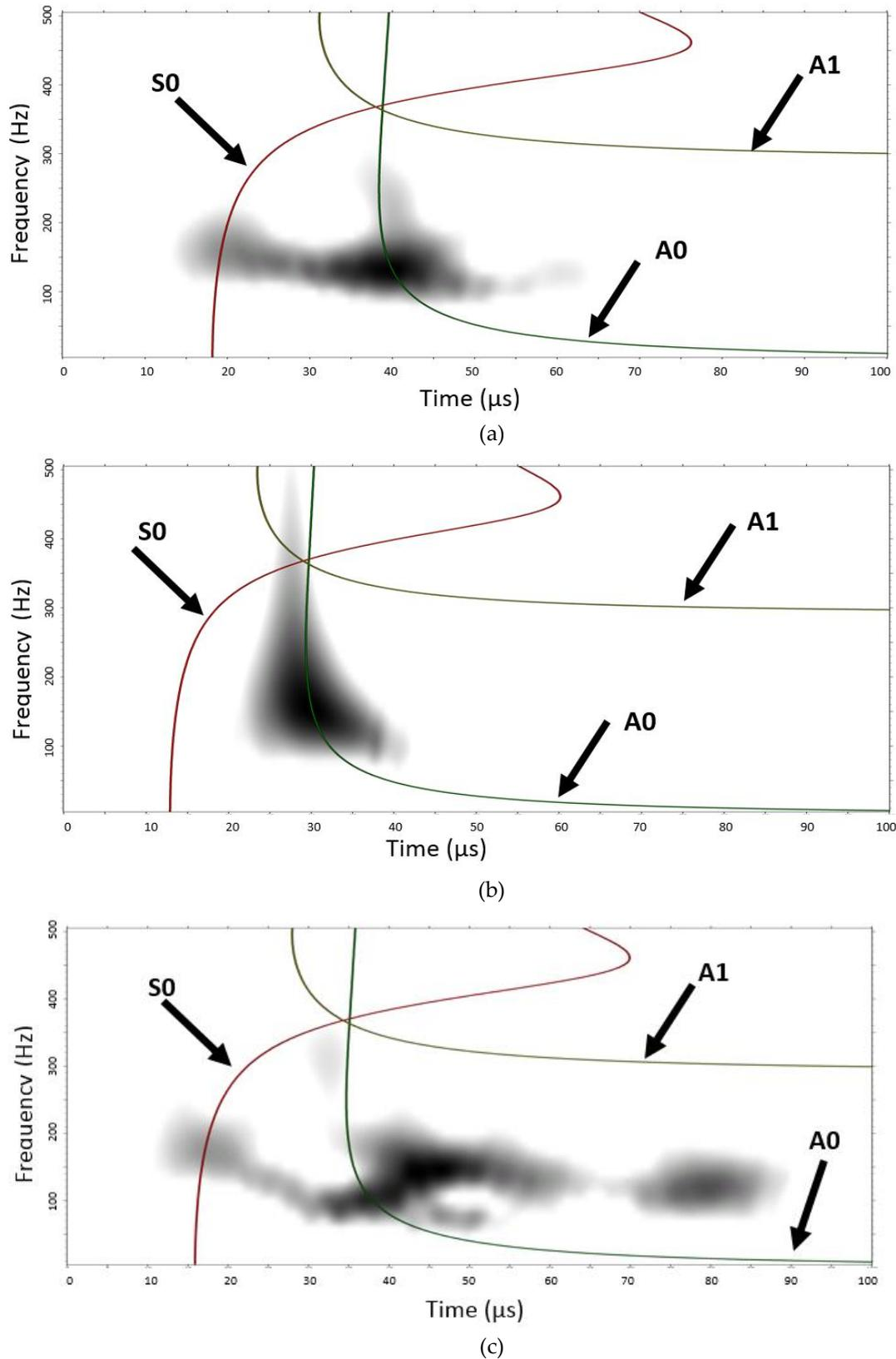
388 **Figure 13.** Superimposed symmetric mode and anti-symmetric modes after converting group velocity
