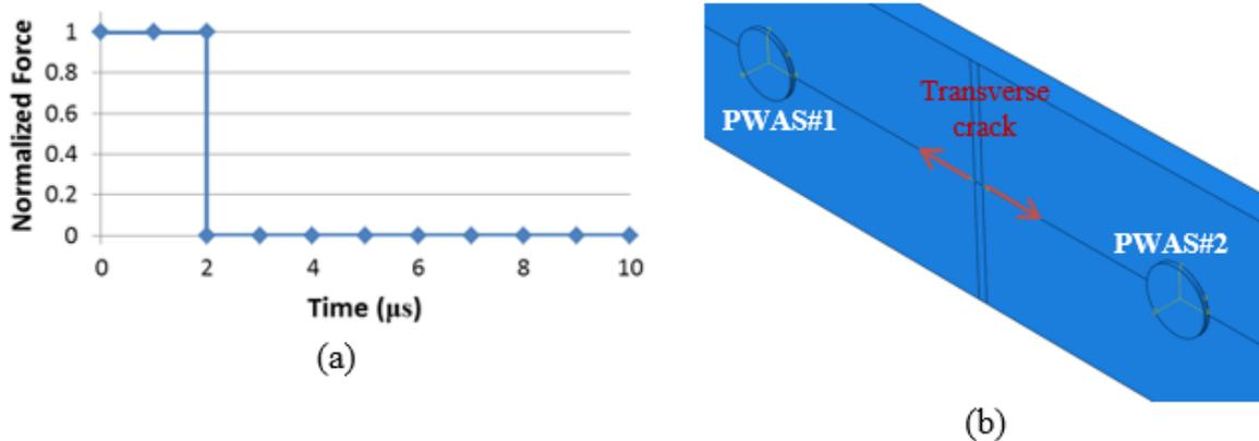
Figure 6. (a) Source function used: at time zero the force step up from 0 to a nominal value 1, and then return to 0 at  $2\mu\text{s}$ ; (b) two-point source force to simulate the energy release by the transverse crack.
