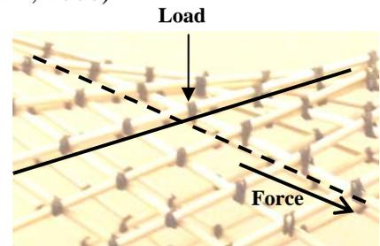
Increasing the diameter at the ends of the structure also increases the tension within it therefore making the whole structure **stiffer** and therefore allowing **longer spans**.
