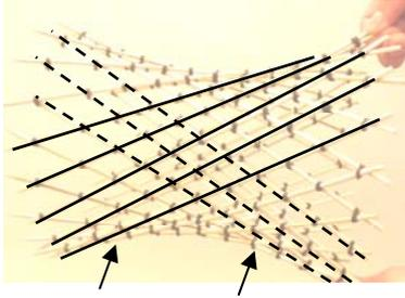
Top beam in compression Lower beam in tension
