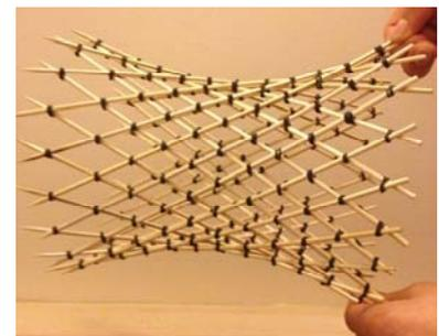
The two opposite curves of the structure create the strength as the bottom curve strengthens and stabilizes the structure by pulling it down. One curve would be weak alone.
