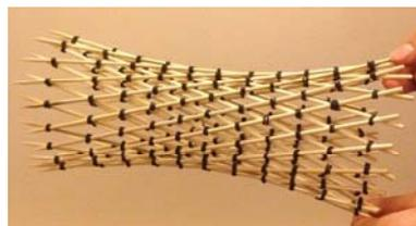
Due to the diagrid nature of the structure, when a force is applied to increase the diameter, the members are forced to twist creating a hyperboloid shape where the centre has a smaller diameter than the ends.
