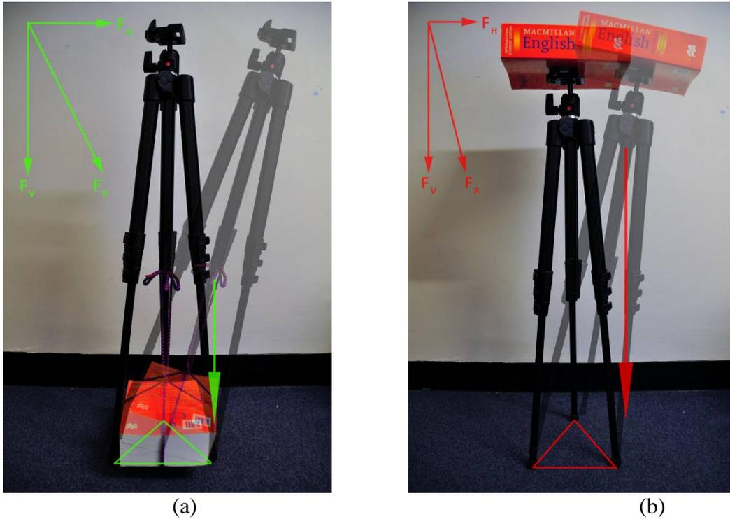
Figure 2: Tripods with different height of centre of mass.
