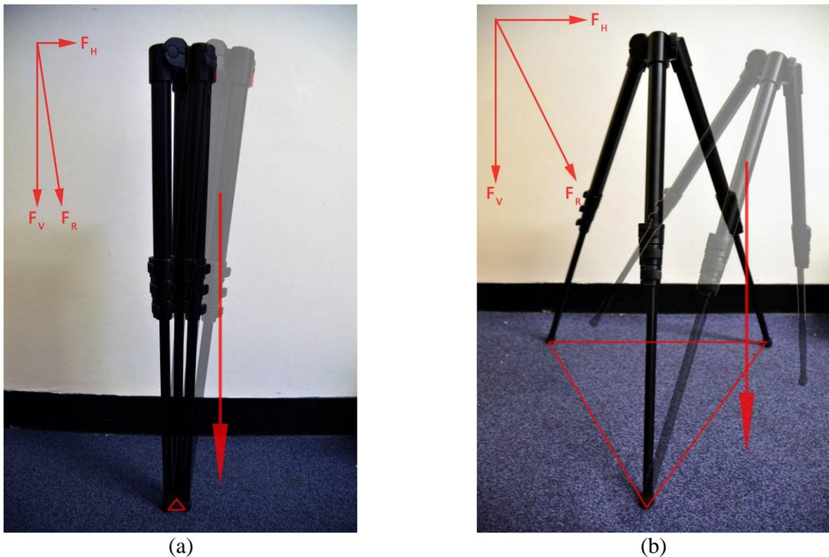
Figure 1: Tripods with different base area.
