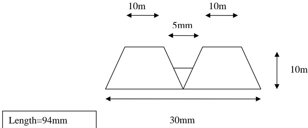
The shape is above undergraduate level so I shall work out the moment of inertia for one finger. Using the above formula and approximate dimensions  $a, c, d = 10\text{mm}$  and  $b = 15\text{mm}$  give the second moment of area to be  $I_{xx} = 3403\text{mm}^4$ .
