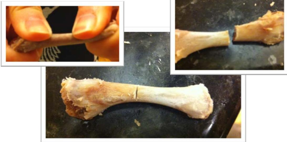
People in China like eating Sparerib Soup, while the ribs are difficult to cut off and snap (see above). A common method to deal with this problem is to use knife to make a crack on the bone. It can be found that just a small bending moment can break the bone into two pieces. Obviously, the crack gives rise to the stress concentration (the stress is higher near the crack than that in other parts of the bone), so it is easy to break the bone.
