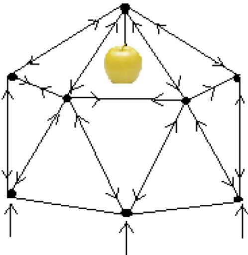
Vertical and horizontal forces are distributed to the foundations through the members in tension or compression.
