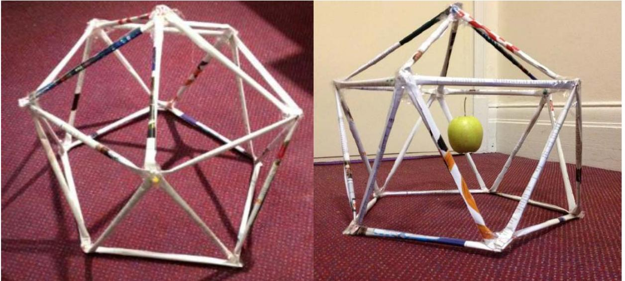
The model consists of wrapped magazine pages of equal size (which are quite good in tension but susceptible to buckling). The members were pinned at each end, forming equilateral triangles.
