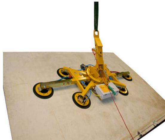
fig 2: Vacuum lifter, lifting a panel
