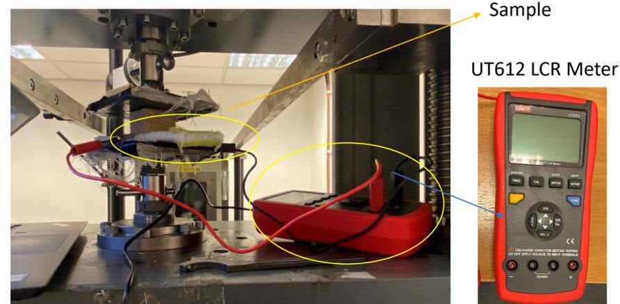
The samples were tested on a Zwick Roell Z50 tensile tester with Wheatstone bridge circuit.
