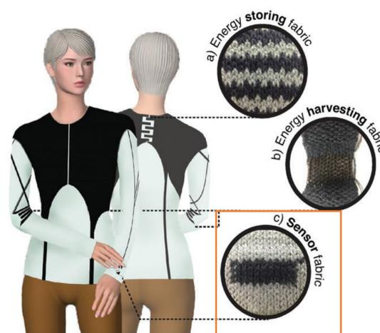
The figure illustrates a garment incorporated with a capacitive touch sensor which responds to variable pressures (Uzun et al., 2019).
