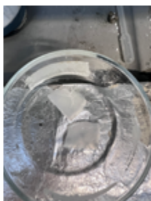
Immersion of the nanofiber membrane in the base solution
