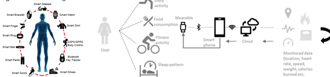
Figure 1 Monitoring system for wearable technology(Arogamam, Manivannan and Harrison, 2019)
